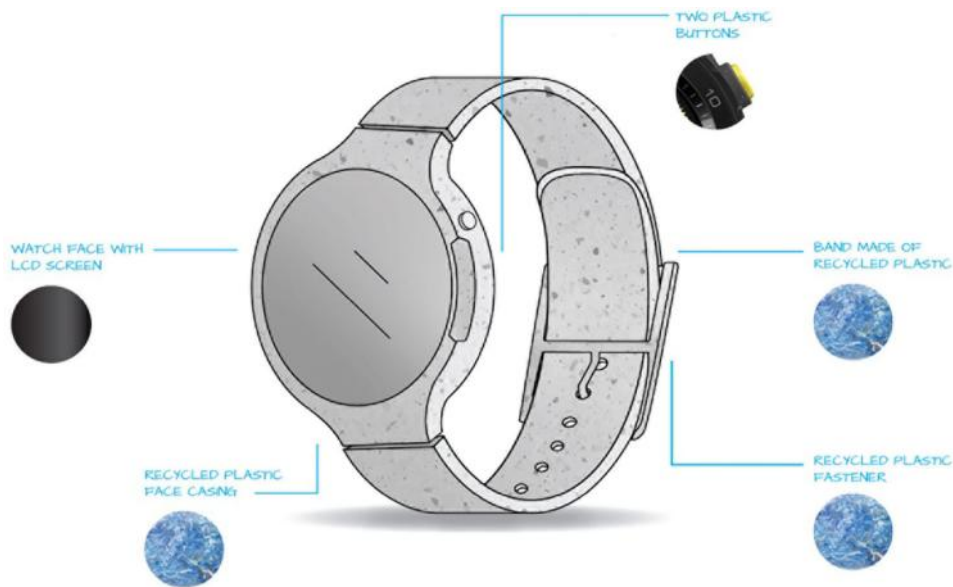
Fig. 2 Eco smartwatch example with a recycled plastic wristband and a complex fastener method
