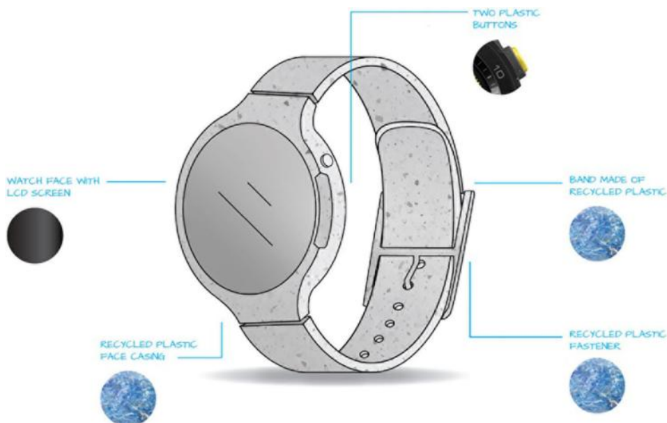
Fig. 6 Option one smartwatch example with a circular screen and a recycled plastic
