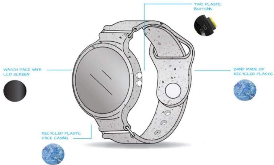
Fig. 3 Uni-Eco smartwatch example with a recycled plastic wristband and a simple fastener method
