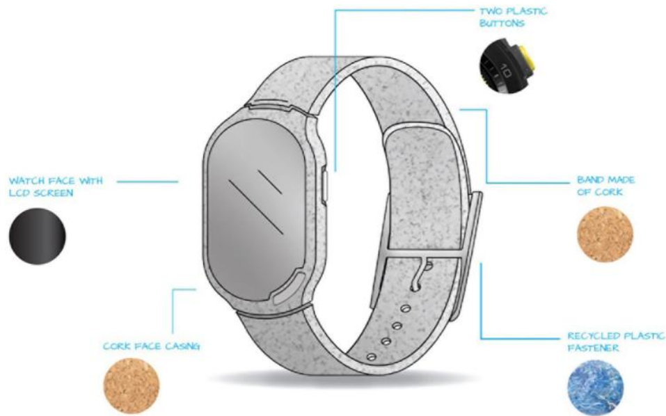
Fig. 7 Option two smartwatch example with an oval screen and a cork wristband
