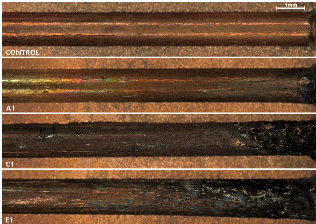
Fig. 2. Digital images of control (factory new), A1, C1, and E1 contact tips.
